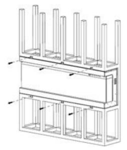
8. Cover the glass panel with protective plastic bag and install plywood or drywall.
