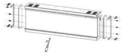
4. Remove the screws from the fireplace as shown in the picture below.
