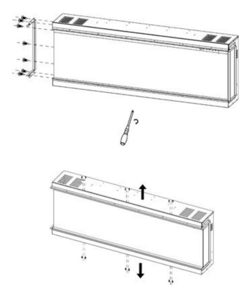
5. Fix the brackets with the screws in the previous step.
