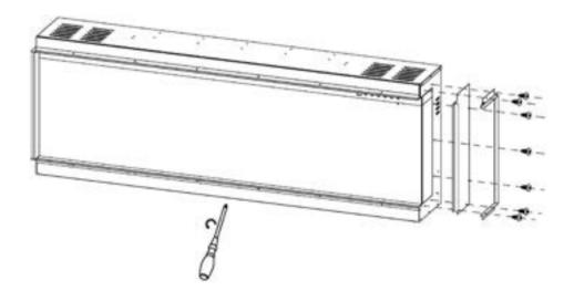
**3.** Fix back the fending bar after the panel is removed.
