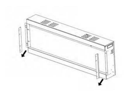
**5.** Place the left and right trims on the appliance and fix the part using the screws provided in the kit.
