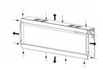
7. Place the top and bottom trims on the appliance and fix them using the screws removed in the previous step.
