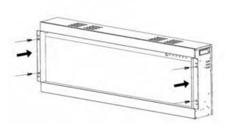
**6.** Remove the relevant screws at the top and bottom of the appliance.
