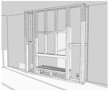
Construct the cavity to the desired size, allowing for the following wall opening dimensions: 1250W x 435H x 254D mm
