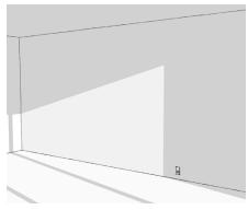
Find a suitable location with an electrical outlet within **1m** of the fireplace.
