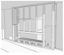
Construct the cavity to the desired size, allowing for the following wall opening dimensions: 1758W x 435H x 254D mm
