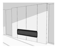
Insert the fireplace into the wall opening and align to the finished wall lining. Fix in place through the side brackets. Protect the glass panel until completion.
